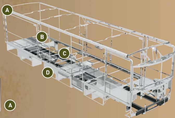
**SUPERSTRUCTURE®** is the term given to Winnebago Industries' structural motor home design and construction. Rather than a single component, it is the culmination of design integration that incorporates steel and aluminum substructures; welded tubular steel floor risers; interlocking joint technology; and Thermo-Panel® floor, roof and sidewalls to form a high-strength, durable vehicle body.
