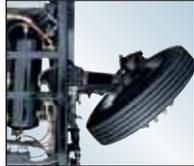
Sharp, 55 degree wheel cut enables superior maneuvering in tight spaces.
